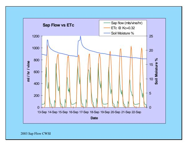
This chart shows an alternative comparison of sap flow vs. ET. The ETc may also be shown in ml/hr per vine by dividing ETo \*Kc per hectare by the number of vines per hectare (2240/hc). Ten representative days are shown here, with sap flow in green, and ETc in orange. The flow rates are shown to decline within two to three days after irrigation. An accurate comparison can be done only with daily totals.
