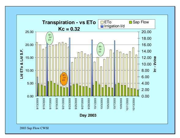
This chart shows the data for an entire month. The data is presented in liters per vine sap flow and liters per vine ETo. The results are similar to the previous chart in mm water use. The analysis process is identical either way.
