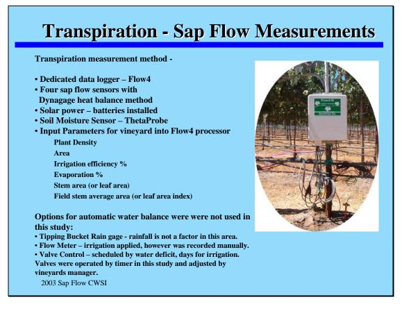
There are two approaches possible for sap flow transpiration stress measurement. One approach would be to compare sap flow by set of well-watered plants with a set of plants in stressed conditions. This method requires two sets of plants and two independent records of sap flow, but could be performed without a weather station reference ETo.
