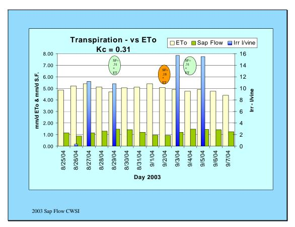
In this chart all the hourly data is converted to sap flow on a daily basis. All the sap flow for 24 hours is added together and multiplied by the number of plants per hectare, then converted to mm depth of water consumption. Irrigation is shown on the right scale in liters per plant. ET is shown as the reference ET provided by the CIMMIS weather station. ET is provided in mm/hr, so it is also added together for 24 hours to provide the daily ETo.
