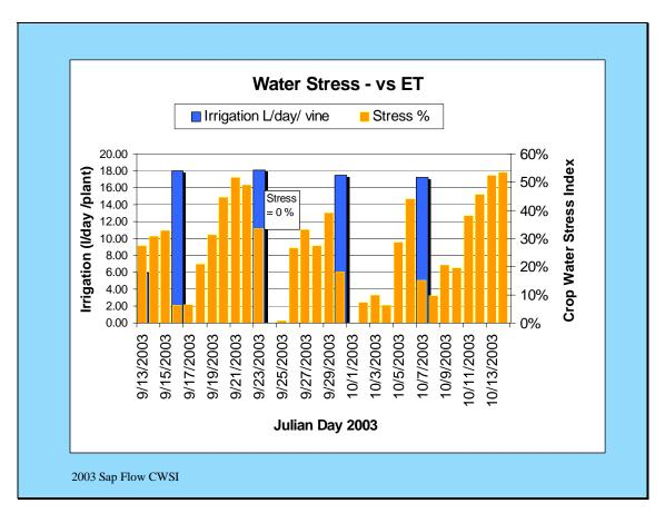
The final analysis of CWSI for 32 days. The average of the daily stress is 25% for the 32 days. This is only slightly different that the stress derived from the total transpiration for the vines (130.9 l) vs. the total ETm (177.3) for the same 32 days. The average stress was 5% more for irrigation once a week, (about 18 l / plant each week), compared to the stress from irrigation twice a week (about 26 l /plant each week).
