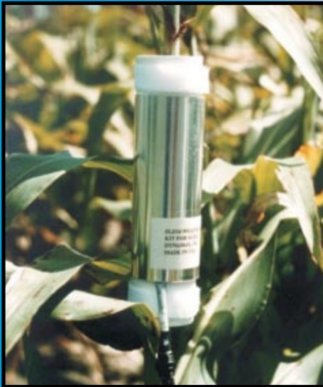
SGB16 sap flow sensor with weather shield attached.
