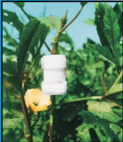
SGA5 microsensor, with weather shield, monitors okra plant transpiration.
