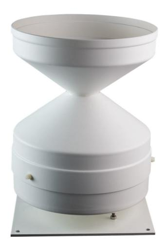
The cost effective ARG100 aerodynamic "tipping bucket" rain gauge has been designed to minimise the established effect of wind on reducing rainfall catch. The benefit of this is more accurate rainfall measurements compared to conventionally shaped rain gauges which catch less than the ARG100.
