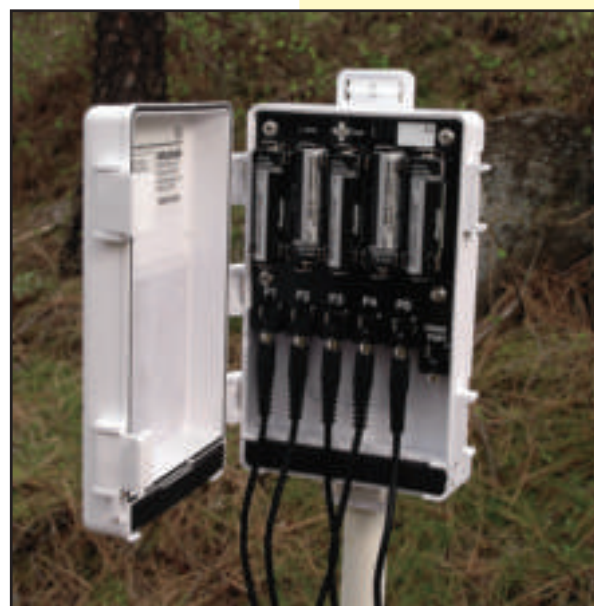
▲ Em50 logger is a turn-key logger for all Decagon's sensors.
